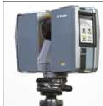
[Fig. 3] Photograph of 3D Scanner
