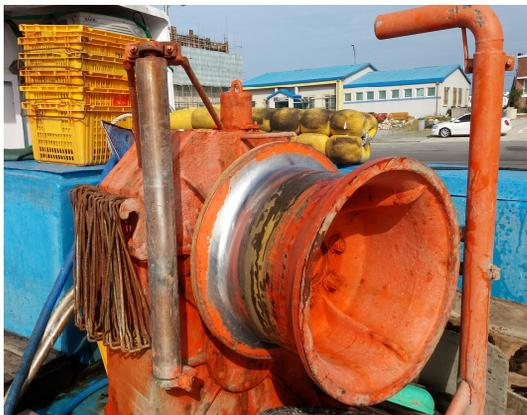
[Fig. 4] Installed hydraulic hauler on the deck of an offshore red snow crab trap fishing vessel.
