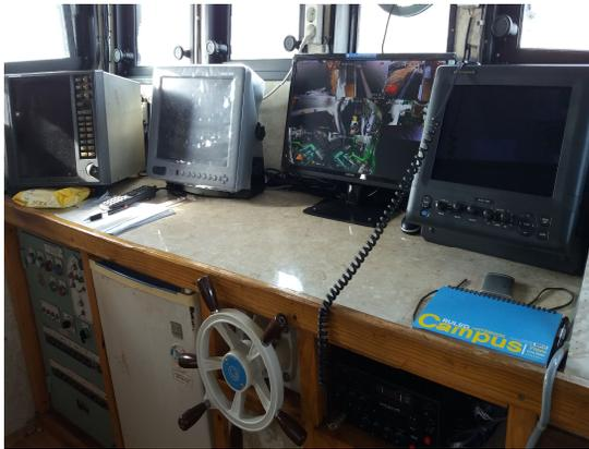
[Fig. 3] Installed navigation equipments in the bridge of an offshore red snow crab trap fishing vessel.
