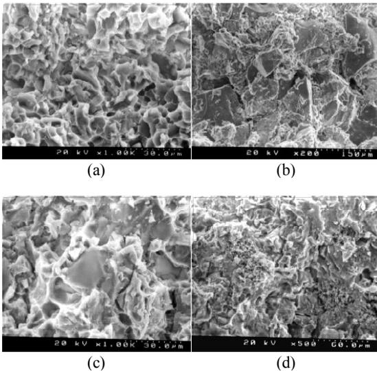
[Fig. 5] Scanning electron micrograph of fractured surface : (a) Al matrix, (b) SiC<sub>p</sub>/Al matrix composites, particle size 100µm, (c) SiC<sub>p</sub>/Al matrix composites, particle size 38 µm, (d) Al<sub>2</sub>O<sub>3p</sub>/Al matrix composite (Vf:40%)
