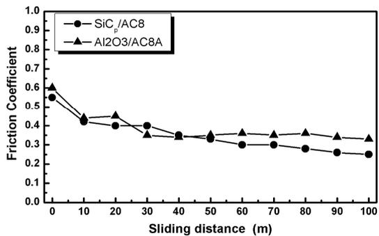
[Fig. 8] Friction coefficient plotted vs sliding distance of SiC<sub>p</sub>/Al matrix composites.
