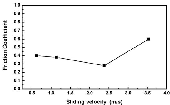
[Fig. 9] Friction coefficient plotted vs sliding velocity of SiC<sub>p</sub>/Al matrix composites.
