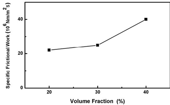
[Fig. 6] Effect of volume fraction on fractional work of Al<sub>2</sub>O<sub>3p</sub>/Al matrix composite.
