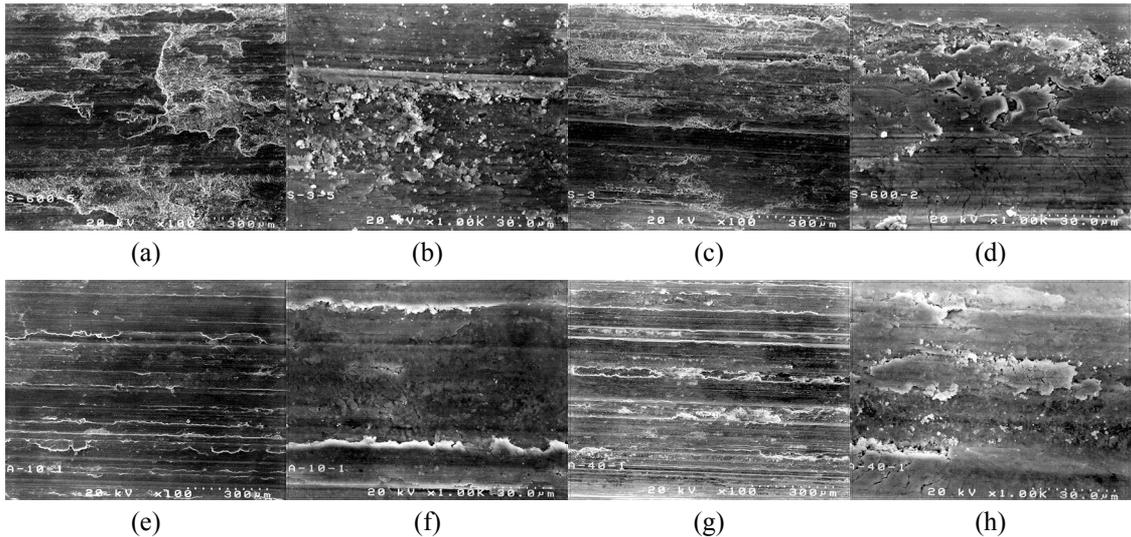
[Fig. 10] Morphology of worn surface : (a) SiC<sub>p</sub>/Al matrix composites at sliding velocity of 0.6 m/s, (b) high magnification of (a), (c) SiC<sub>p</sub>/Al matrix composites at sliding velocity of 3.53 m/s, (d) high magnification of (c), (e) Al<sub>2</sub>O<sub>3p</sub>/Al matrix composites at sliding velocity of 0.6 m/s, (f) high magnification of (e), (g) Al<sub>2</sub>O<sub>3p</sub>/Al matrix composites at sliding velocity of 3.53 m/s, (h) high magnification of (g).
