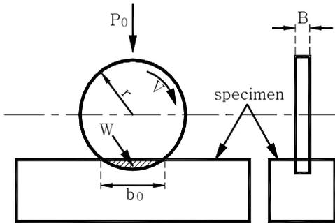
[Fig. 2] Schematic wear tester
