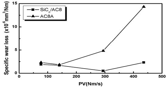
[Fig. 3] Effect of Pv factor on wear loss of SiC<sub>p</sub>/Al matrix composite and Al matrix.
