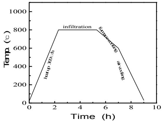
[Fig. 1] Processing temperature cycle for fabrication of composites
