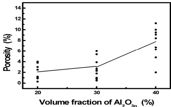
[Fig. 7] Porosity level of Al<sub>2</sub>O<sub>3p</sub>/Al matrix composite with volume fraction.
