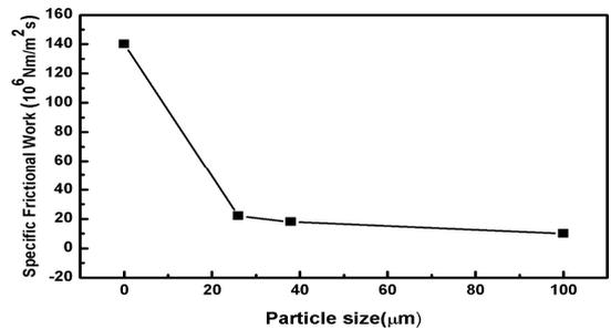
[Fig. 4] Effect of reinforcement particulate size on fractional work of SiC<sub>p</sub>/Al matrix composites.
