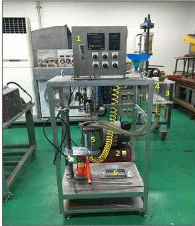
[Fig. 1] A picture of experiment device (1. Control Box 2. Air Compressor 3. Solution Storage A 4. Solution Storage B 5. Mixer 6. Mold).
