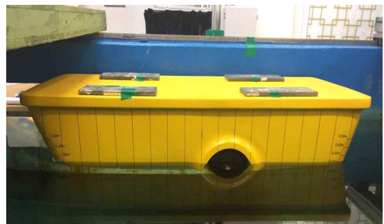
[Fig. 3] Inclining test of Model ship
