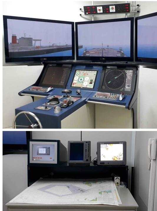
[Fig. 1] Navigation equipments used in the wheelhouse for radar simulation training
