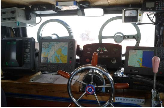
[Fig. 2] Navigation equipments in the wheelhouse of 5 tons coastal composite fishing vessel
