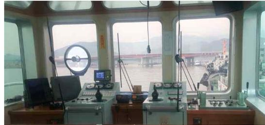
[Fig. 4] Navigation equipments in the wheelhouse of 292 tons tugboat
