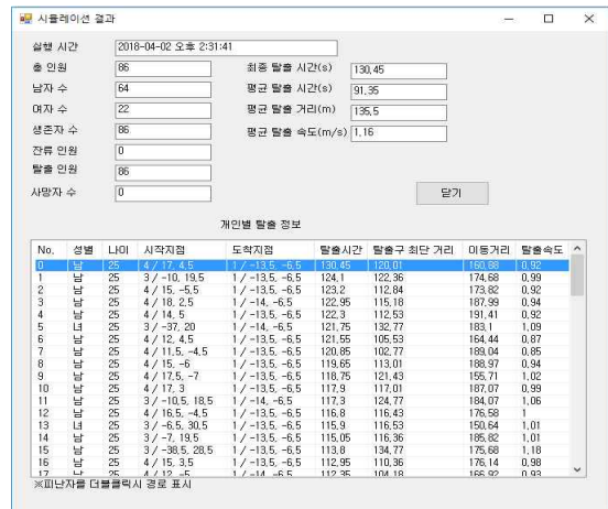
[Fig. 6] Analysis of Evacuation simulation result (abandonship drill).
