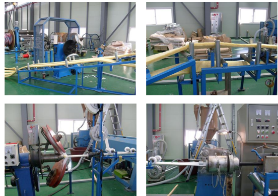
[Fig. 2(a)] Photo of the process of multi core tube Continued wrapping glass wool and tapping process
