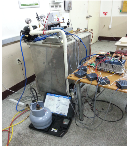
[Fig. 2] Refrigerant filling of experimental device (R1234yf)
