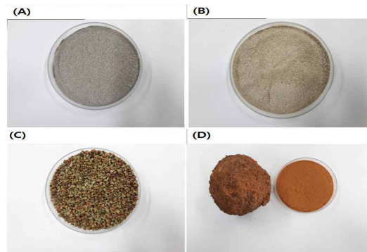
[Fig. 1] Appearance of remediation materials; (A) Abalone shell powder, (B) Oyster shell powder, (C) Cleanlite, (D) EM soil ball.
