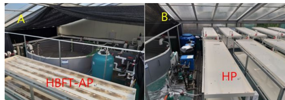
[Fig. 1] Compartments and water flow of the experimental design: (A), HBFT-AP (hybrid biofloc technology-aquaponics) system: fish tank (ø 4.5 m) → sump tank (2×1 m) → pump (1.5 HP) → biohelix filter(680 L) → vegetable bed (2.9×0.6×0.1 m, No. 20) → fish tank; (B), HP (Hydroponics): nutrient solution tank → pump (1 HP) → sump tank (1×0.5×1 m) → pump(1.5 HP) → vegetable bed (2.9×0.6×0.1 m, No. 20) → sump tank. Lee et al. (2019b).
