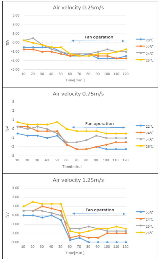
[Fig. 6] Relationship between TSV time series and room temperature at set air velocity.
