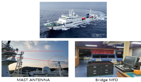
[Fig. 6] Radar Installation.
