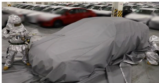
[Fig. 6] Suffocation fire blanket for EVs-fire (source: hyundai glovis).
