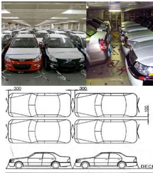
[Fig. 8] Vehicle loading and lashing plan of PCTC source: development for loading optimization and ship operation safety support service for vehicle carriers(2017).
