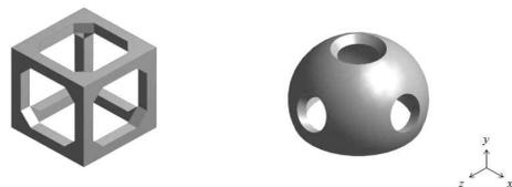
[Fig. 2] Target artificial reefs: a cube-type reef (left) and a half-ball type reef (right)
