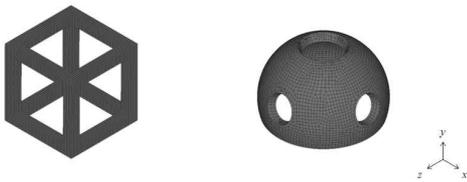
[Fig. 3] Finite element models of cube-type reef (left) and half-Ball type reef (right)
