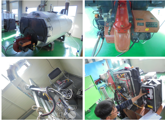
[Fig. 2] FNB-100(2) Gun-type Burner Assembly.
