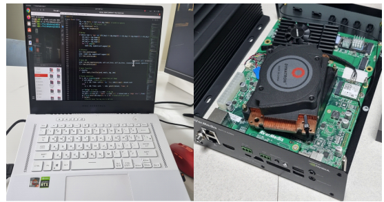
[Fig. 2] Hardware for system base on edge computing: laptop and Jetson Xavier AGX.
