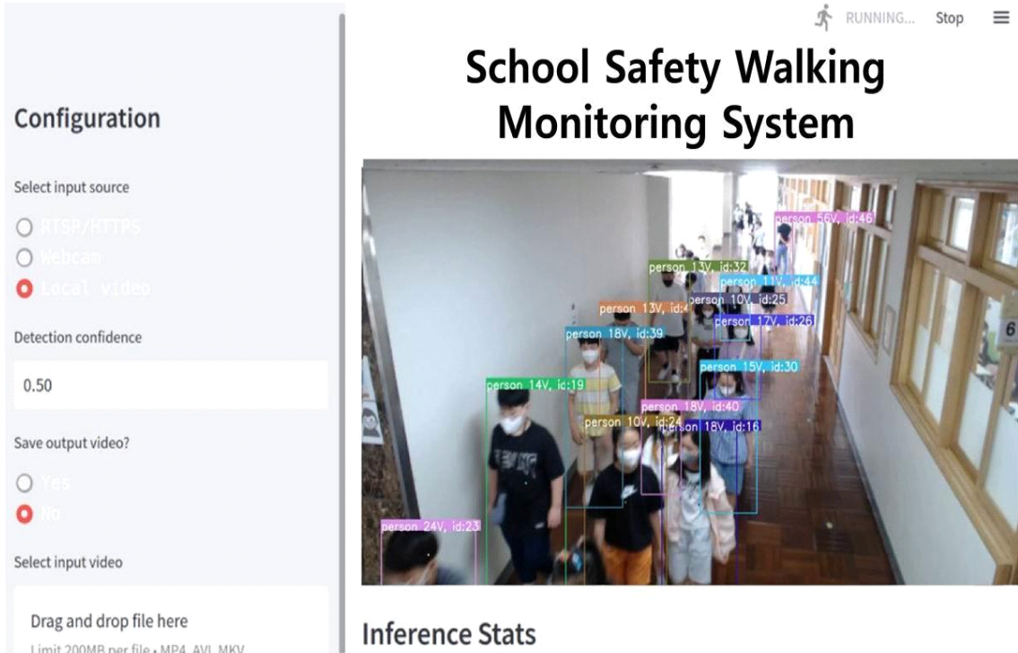
[Fig. 9] Dashboard of school safety system for pedestrian applied Streamlit.
