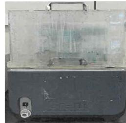
[Fig. 3] Immersion corrosion test setup following ASTM G31-21 standard.
