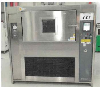
[Fig. 2] Cyclic corrosion test equipment(CCT-1LZ) used for the experiment.
