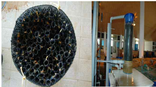
[Fig. 2] Photos of Small-scale degasser Equipment and Tubular packing media
