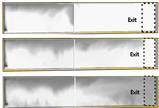
[Fig. 8] Visibility distribution of fire door (23, 50, 100sec).
