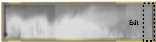
[Fig. 5] Visibility distribution without draft curtain.
